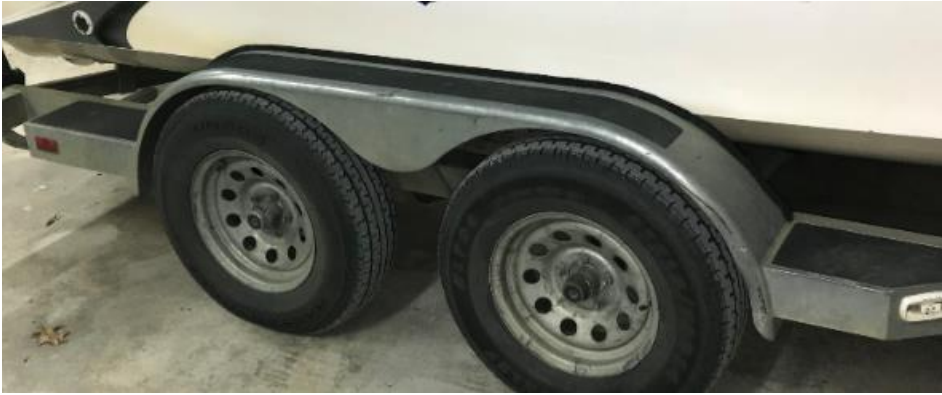
Picture #1: Heavy duty fenders with step locations on each side for easy access into boat.
