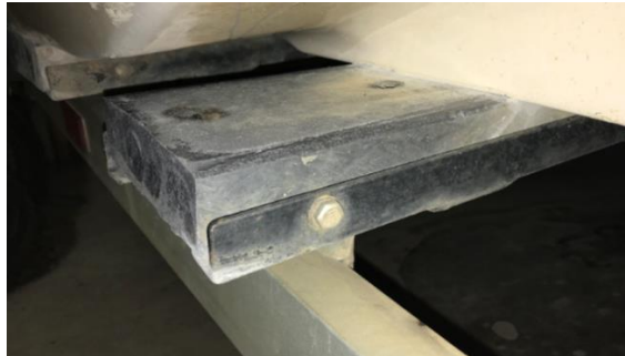
Picture #3 & #4: Reinforced boat trailer bunk with polyethylene type material for bunk.
