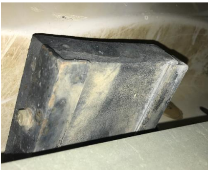
Picture #2 & #3: Reinforced boat trailer bunk with polyethylene type material for bunk.
