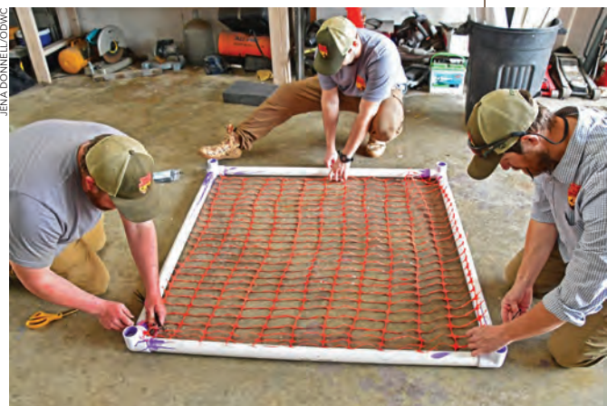
Employees attach orange snow/safety fencing to the bottom of a fish habitat cube as part of the construction process.
