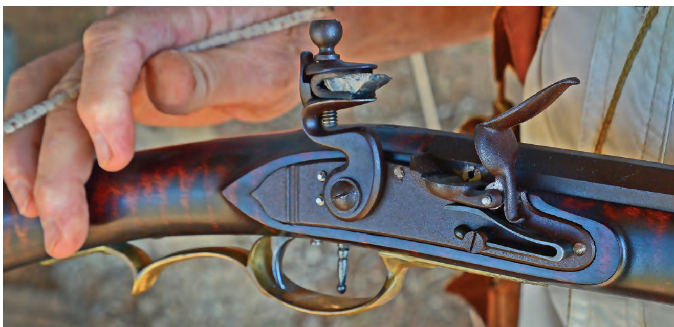
This view clearly shows the flint in the flintlock.
