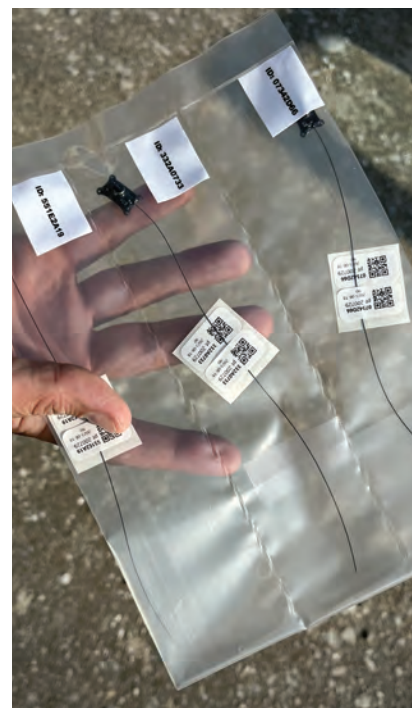
Motus tags like these are attached to animals and detected by the receiver network, allowing biologists to track animal movement.
