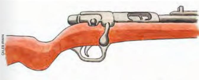
The bolt action is most often seen in rifles. Bolt action firearms are common and simple to use. Opening a bolt action firearm is as simple as pivoting the bolt upwards and pulling it backwards, using the handle on the bolt.
