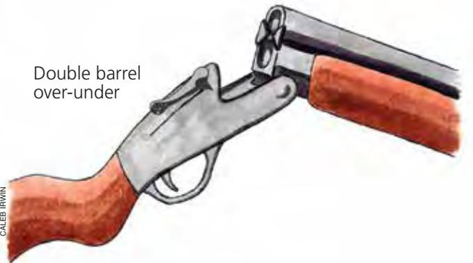
The action release on a break action firearm is usually on the top of the firearm behind the chamber.
