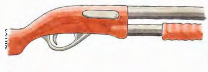
The pump action is more commonly seen in shotguns than in any other type of firearm. It is a very reliable action, and an experienced shooter can go through the pumping actions very quickly, and instinctively. Sliding the front grip back and then forward ejects the spent shell, loads another shell and cocks the hammer.
