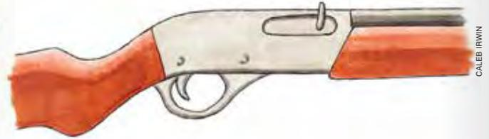
The semi-automatic action is very popular in both rifles and shotguns. A semi-automatic fires a bullet, ejects the spent cartridge and chambers a fresh cartridge each time the trigger is pulled.
